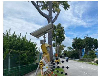
Solar panel for robotic traffic controller
